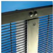
**Angle Iron Posts:** Posts are 70 x 70 x 6mm / 100 x 75 x 8mm (3000mm panel) are hot dipped galvanized in accordance with ISO-1461 and pre-drilled with holes for fixing panels, including (70 x 6mm) cover plate section with pre-drilled holes for fixing panels to posts. The panels are fixed to posts using stainless steel (M8 x 40mm) countersunk flushlock bolts and shear nuts.
